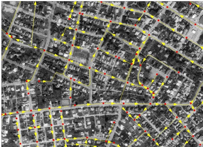
USGS DOQ_Q Image as a Basemap for Sanitary Sewers and Manholes
